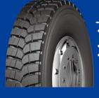
Optimized tread block pitch sequence offers Optimized design to reduce noise generation
